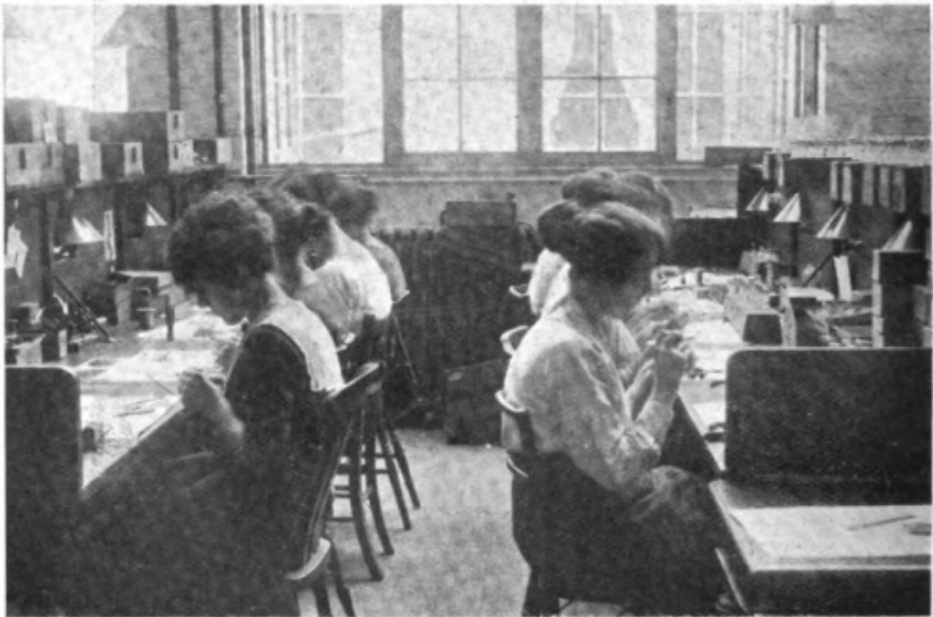
An assembling bay, where filaments, grids and plates are fitted.
