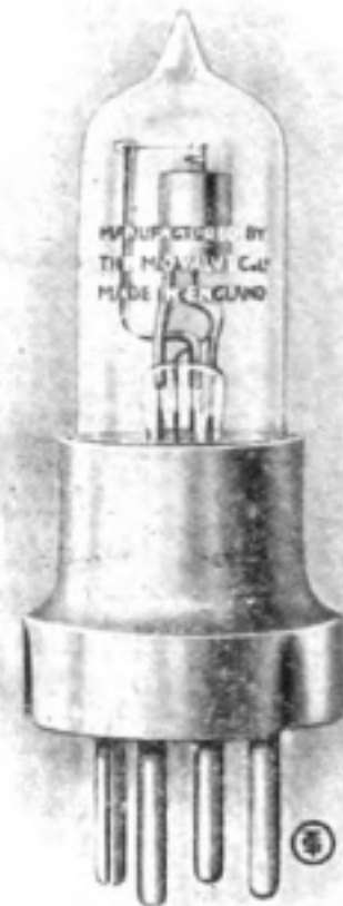
Low Temperature Emitter, Type L.T3. Requires a filament potential of only 1.8 volts and passes a current of 0.11 amperes. An efficient detector, oscillator, high and low frequency amplifier.
