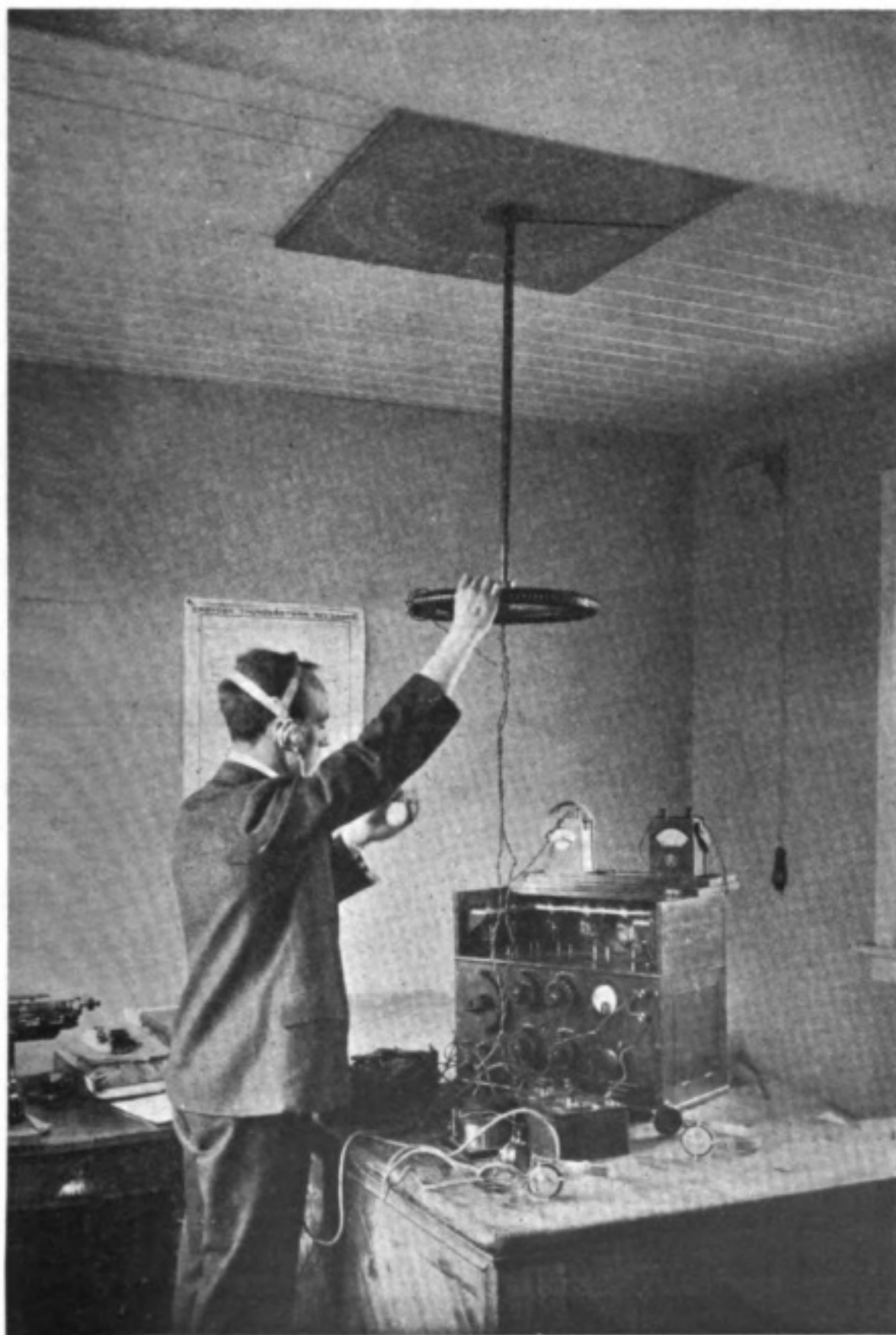
Fig. 2. Croydon Aerodrome Meteorological Station. "Atmospheric" D.F. Apparatus, or "Thunderstorm Finder"—an auxiliary investigation carried out in the field of meteorology by means of wireless.
