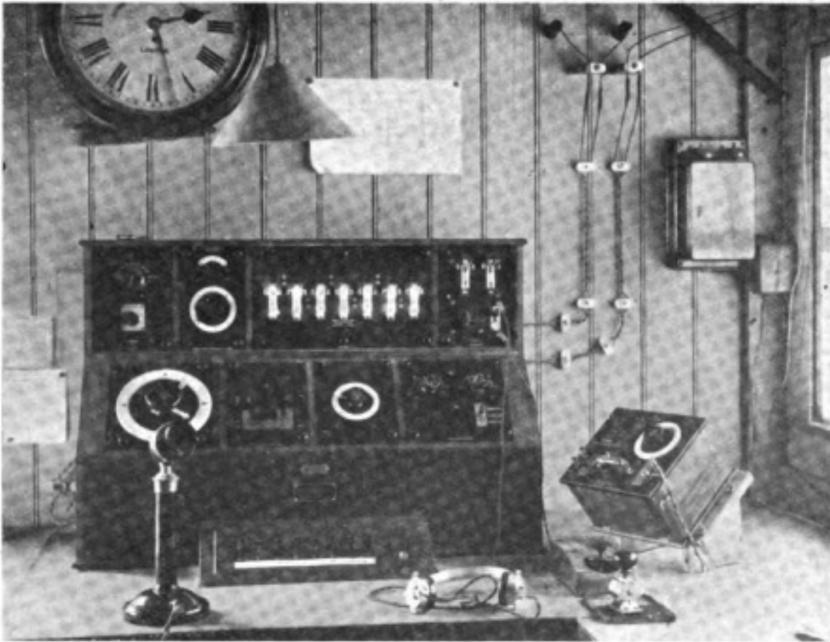
Fig. 2. The Direction Finder and Receiver.
